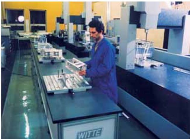
Loading station for 3 CMMs with transfer bridges for pallet exchange
