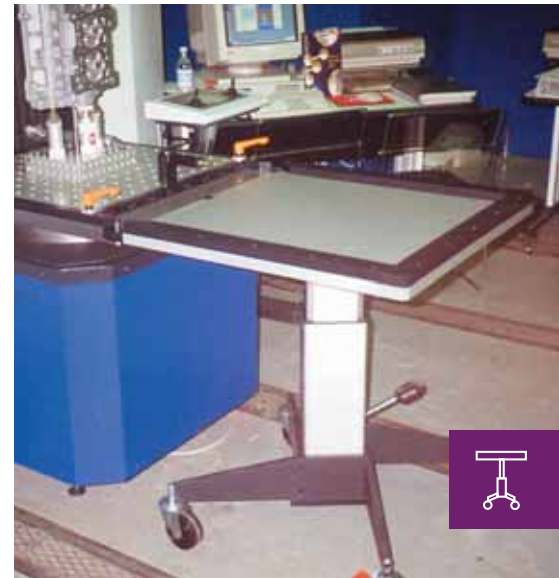
Jack up trolley #81945 used with a CMM
