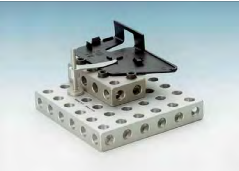
Workpiece set up on screw-jacks and secured with hold down springs
