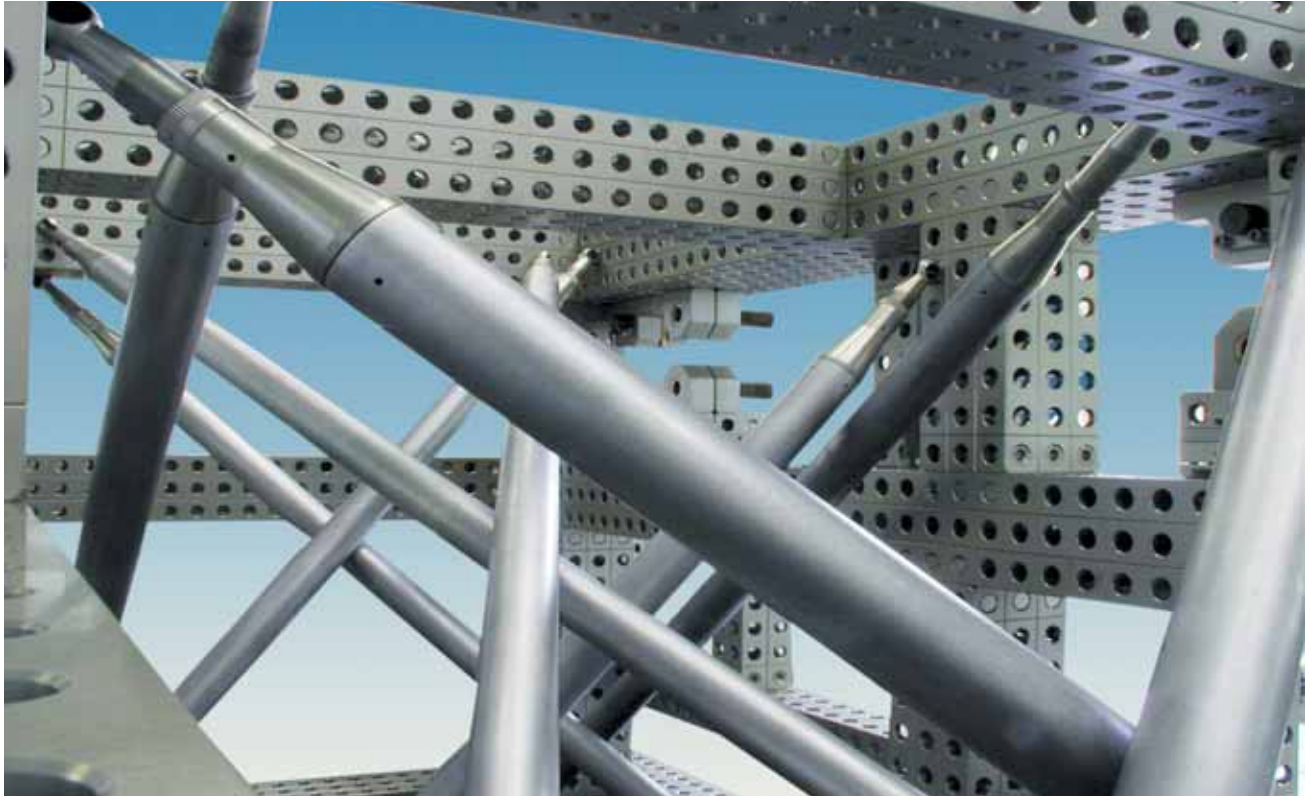
Application example: Universal struts used crosswise
