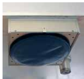
Hovercraft cushion cassette shown on underside of plate
